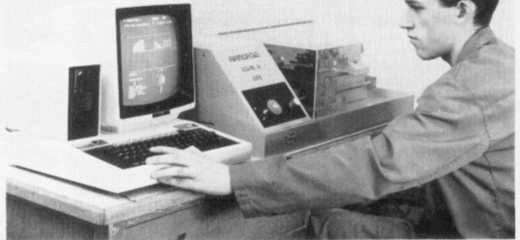
The BBC Micro controlling a small lathe
